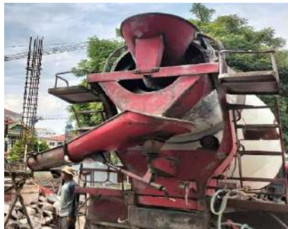
Gambar 4.8 Beton Ready Mix
